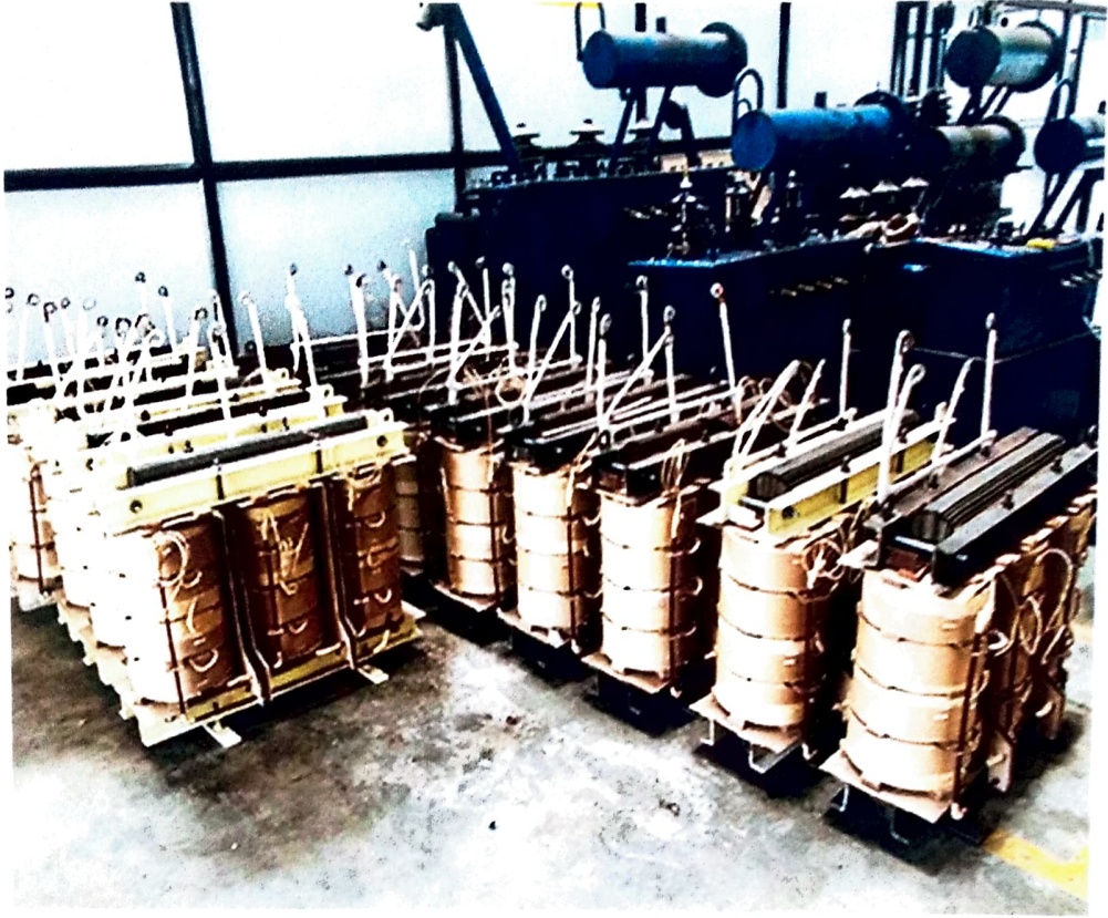
Photo 5: Types of Core Assembly
