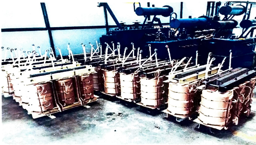
Photo 4: Types of Core Assembly
