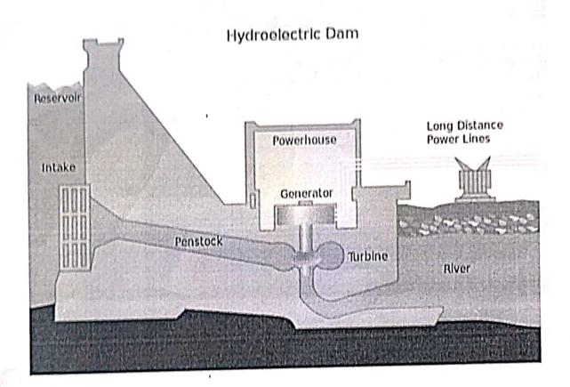
Today, modern hydro plants produce <u>electricity</u> using turbines and generators, where mechanical energy is created when moving water spins rotors on a turbine. This turbine is connected to an electromagnetic generator, which produce <u>electricity</u> when the turbine spins.
