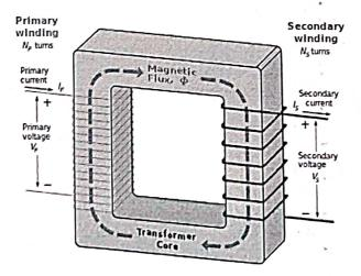
A static electrical machine used for transforming power from one circuit to another circuit without changing frequency is termed as Power transformer. The transformers are generally used to step down or step up the voltage levels of a system for transmission and generation purpose. These transformers are classified into different types based on their design, utilization purpose, installation methods
